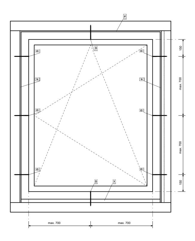
Attachment points of the blaugelb Triotherm+ pre-wall installation system – combined diagram
